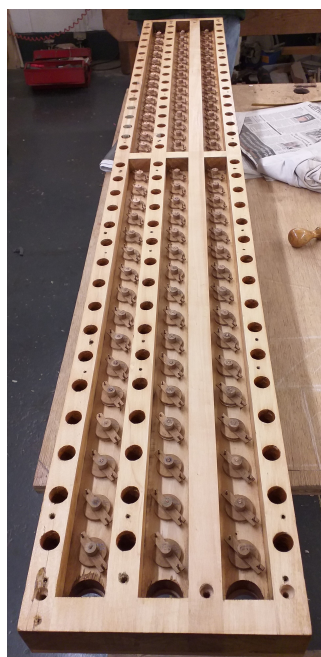
The restored main chest of the 72-key Decap is seen above. As well as re-leathering, all the threaded valve wires have been replaced. The melody and counter-melody sections are separated in the middle, resulting in each division having three registers, each of 16 playing notes.
