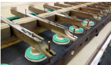
Detail of a restored windchest incorporating Marengi's lever action.
