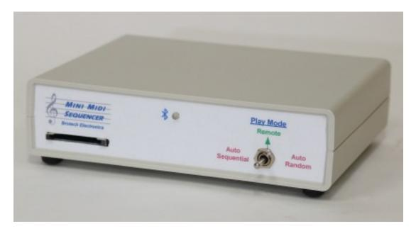
The front of the Mini Midi Sequencer+, showing (on the left) the SD card slot, and on the right the play mode selection switch. In the centre is the bi-colour Bluetooth status indicator.
